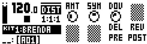
**AMT** (Distortion Amount) controls the amount of distortion applied to the signal. Range (0-127).
