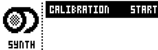
**CALIBRATION** will start the calibration routine for the oscillators and filters. After selecting this option, a popup window asking to confirm the calibration will appear. Press **[YES/SAVE]** to proceed with the calibration. Please note that the calibration routine takes a while to complete.
