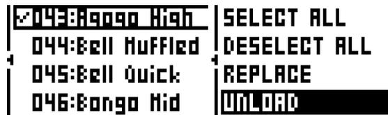
Any sample in the RAM may be individually replaced. Simply highlight the slot containing the sample you wish to replace, open the right hand menu by pressing [RIGHT] and select REPLACE. Browse the directories of the +Drive, locate the desired sample and press [YES/SAVE] to place it in the previously highlighted sample slot. If you wish to go back to browsing the +Drive storage directories, press [LEFT] twice and select VIEW +DRIVE.
