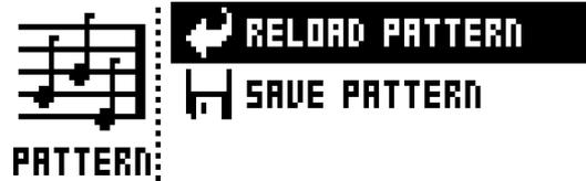
**RELOAD PATTERN** will reload the active pattern. It will either be reloaded to its original auto-saved state or to a specific saved state which can be determined by utilizing the **SAVE PATTERN** command. Press **[NO/RELOAD]** + **[SCENE]** for a shortcut to the **RELOAD PATTERN** command.
