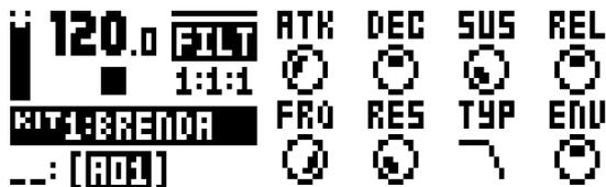
**ATK** (Attack Time) controls the attack time of the filter envelope. Range (0-127).
