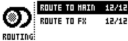
**ROUTE TO MAIN** highlight this option to customize which of the 12 tracks will send to the main output. Use the **[PADS]** to activate/deactivate send from the track of each corresponding pad. **<PADS>** of a green color send to main. Unlit **<PADS>** do not. Note that each track will still send to its individual output.
