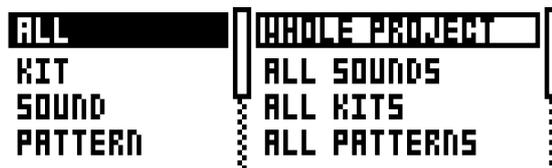
The column to the left selects what will be backed up. Select the column using the **[LEFT]** arrow key. Use the **[UP]**/**[DOWN]** keys or the **LEVEL** knob to scroll through the column. The SysEx data send alternatives located
