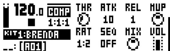
**THR** (Threshold) sets the threshold of the compressor. Lower threshold means a larger portion of the signal will be subject to compression. There is a bar on the rightmost edge of the LCD screen which will visually represent the amount of compression. Range (0-127).
