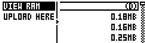
Select VIEW RAM and press [YES/SAVE]. A list will appear, showing all 127 user sample slots. A circle at the very right end of the row means that the sample is currently unused in the active project.
