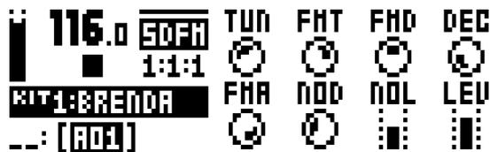
**TUN** (Tune) sets the pitch of the first (modulated) oscillator. Range (-64-+63).
