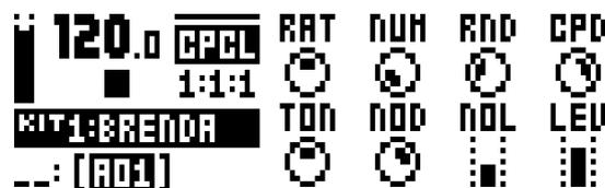
**RAT** (Clap Rate) sets the rate of the initial claps. Range (0-127).
