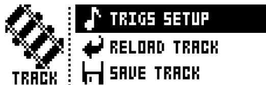
**TRIGS SETUP** will take you to the quantization menu for the active track. See section “QUANTIZATION” on page 38.
