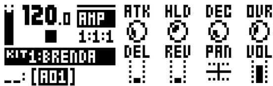
**ATK** (Attack Time) controls the attack time of the amp envelope. Range (0-127).
