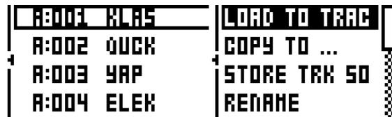
**LOAD TO TRACK** loads the selected Sound to the active track and makes it a part of the active kit.
