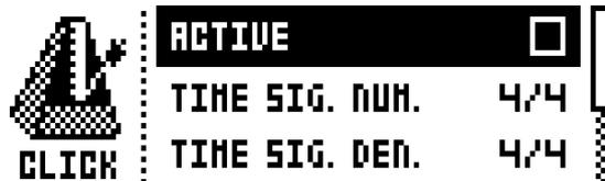
**ACTIVE** activates/deactivates the metronome. It is also possible, outside of this menu, to keep **[FUNCTION] + [RETRIG]** pressed for a second to toggle the metronome click on or off.
