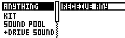
The column to the left selects what will be received. Select the column using the **[LEFT]** arrow key. Use the **[UP]/[DOWN]** keys or the **LEVEL** knob to scroll through the column. The SysEx data receive alternatives located in the column to the right will change depending on the selection made in the left column. Press the **[RIGHT]** arrow key to access this column. Use the **[UP]/[DOWN]** keys or the **LEVEL** knob to select what will be
