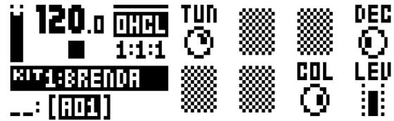
**TUN** (Tune) sets the pitch of the six oscillators of the open hihat. Range (-64-+63).
