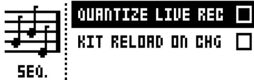
**QUANTIZE LIVE REC** will when active quantize notes entered in LIVE RECORDING mode to complete sequencer steps. When the setting is deactivated, live recorded notes will where applicable be affected by micro timing. Read more about micro timing in the section “TRIG MENU” on page 37.
