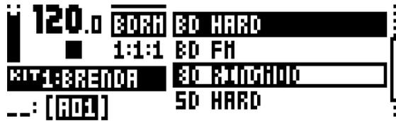
Browse through the MACHINE list using the [ARROW] keys [UP] and [DOWN]. Sample the MACHINE currently outlined by tapping the pad of the active track. Select the outlined MACHINE by pressing [YES/SAVE]. Exit without switching MACHINE by pressing [NO/RELOAD].
