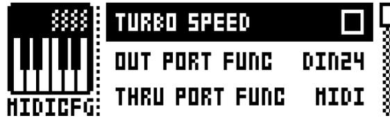
**TURBO SPEED** press [YES/SAVE] to start the turbo speed negotiation. Speed is chosen automatically.
