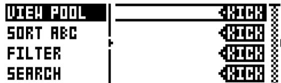
Pressing **[RIGHT]** will access the SOUND OPERATIONS menu. The available operations will affect the high-lighted Sound. Press **[YES/SAVE]** to apply the commands to the selected Sound. Press **[NO/RELOAD]** or the **[LEFT]** arrow key to exit the menu.
