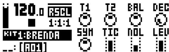
**T1** (Tune Osc1) sets the pitch of the first oscillator. Range (-64-+63).
