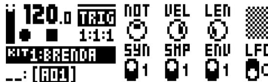
**NOT** sets the pitch of the note when triggered, ranging from -24 to 24. When LIVE RECORDING and playing in CHROMATIC mode, the pitch of the **[PADS]** played will override this setting.
