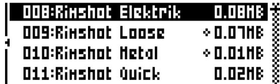
On this screen, the 127 user samples may be unloaded individually or collectively in order to empty the slots. Scroll the list using the [ARROW] keys [UP]/[DOWN] or the *LEVEL* knob. Press [YES/SAVE] to tick individual samples, or bring up the right hand menu by pressing [RIGHT] and choose SELECT ALL. On the right hand menu, select UNLOAD to empty the slots of the ticked samples.
