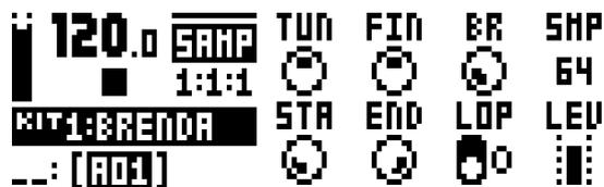
**TUN** (Tune) sets the pitch of the sample in equivalents of chromatic semitones. To move faster, press the knob while turning it. The knob works in a bipolar fashion, with 0, north, leaving the pitch unchanged. Range (-24-+24), equivalent to four octaves.
