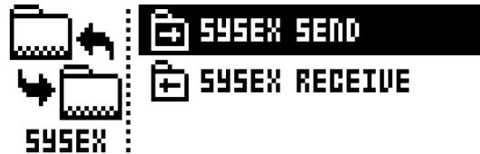
When receiving or sending SysEx data, the MIDI ports or the USB port of Analog Rytm must be connected to the external sending/receiving device.
