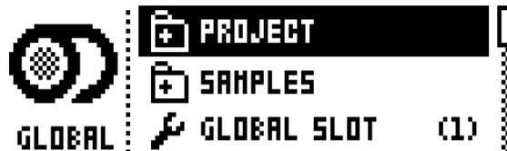
Scroll through the list by using **[UP]/[DOWN]** or the *LEVEL* knob and select PROJECT. Open the menu by pressing **[YES/SAVE]**.
