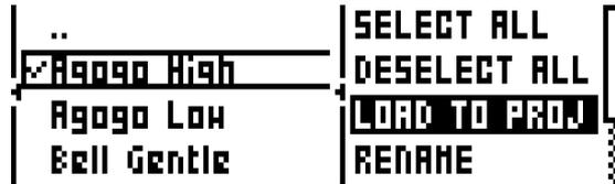
Select LOAD TO PROJECT and press [YES/SAVE]. The samples you selected (ticked) will now appear in the first available empty slots out of the 127 user sample slots of the active project. To view the user samples currently in the RAM of the active project, press the [LEFT] arrow key twice. This will bring up the left side menu.
