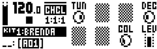
**TUN** (Tune) sets the pitch of the six oscillators of the closed hihat. Range (-64-+63).
