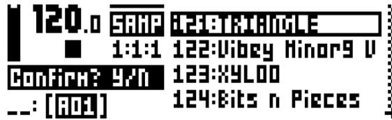
Turn the knob counter-clockwise to scroll up the list, clockwise to scroll down the list. Tap the pad of the active track while browsing to listen to the sample currently outlined.
