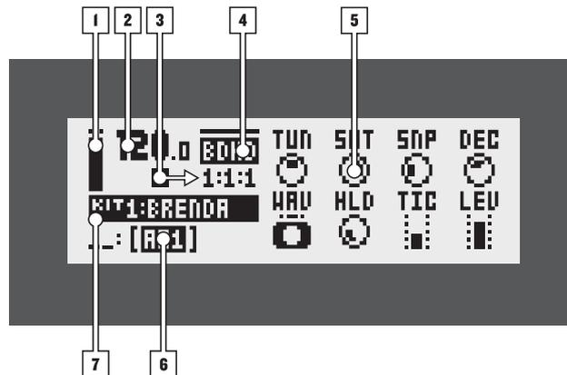
1. Bar showing the main volume setting of the active track. Turn **LEVEL** knob to change.
