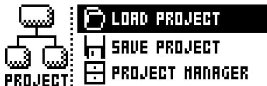
**LOAD PROJECT** opens a project selection screen where you choose a project to be loaded. Note that the active project will not be saved before loading the new project. This menu can be accessed directly by pressing and holding **[FUNCTION] + [TRACK]** for a little while. If you wish to create a new project, select **CREATE NEW** at the very bottom of the list. The new project will be a blank slate.
