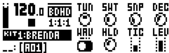
**TUN** (Tune) sets the pitch of the voltage controlled oscillator in chromatic semi-tones. To move faster, press the knob while turning it. Bipolar knob range (-64-+63).
