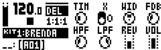
**TIM** (Delay Time) sets the delay time. It is relative to the current BPM and is measured in 128th notes. For instance, a setting of 32 equals a one beat delay (four sixteenth notes). Range (1-128).
