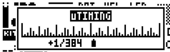
Set the retrig speed by pressing and holding the [TRIG] key while pressing [ARROW] keys [UP] or [DOWN]. Similarly, a pop up menu will appear on the screen, where various retrig settings can be made. Read more about the retrig menu on page 35.
