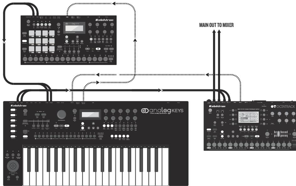
Analog Rytm gets along with other broods of the Elektron breed. Here, it is used with an Octatrack and an Analog Keys.
