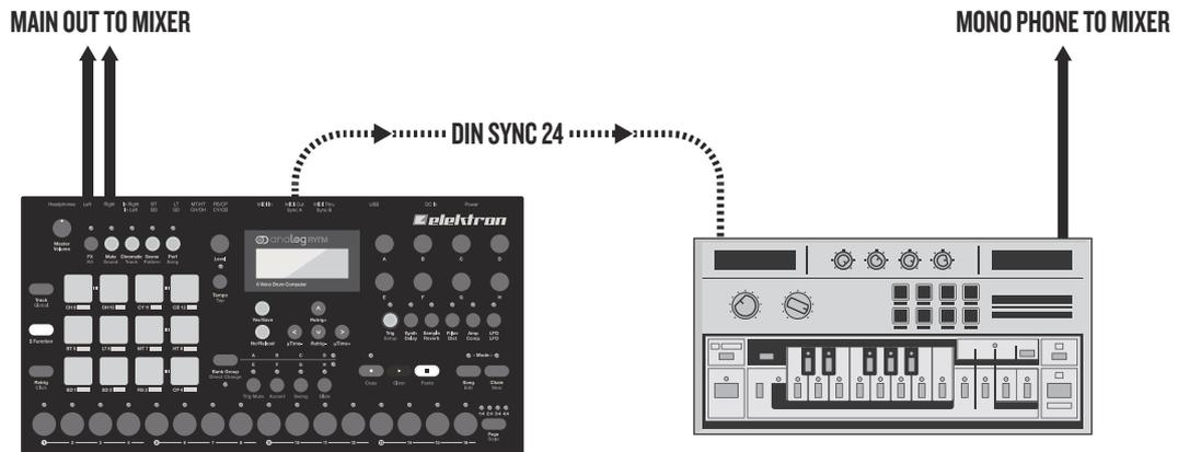
The DIN sync capabilities of the Analog Rytm allows you to use gear from times gone by.
