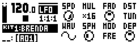
**SPD** (Speed) controls the speed of the LFO. It is synced to the BPM. For the LFO to be synced to straight beats, try settings of 8, 16 or 32. The knob is bi-polar. The LFO shape can be played backwards by using negative values. Range (-64-+63).
