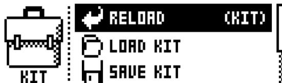
**RELOAD KIT** will reload either the active kit, reverting it to its saved status, or all kits. Using the **[LEFT]** and **[RIGHT]** keys selects whether only the active kit or all kits will be reloaded. **[NO/RELOAD] + [KIT]** offers a shortcut to reloading the active kit.
