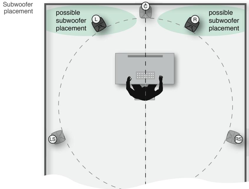
Step 2 Placing the subwoofer to a corner or near the front wall boosts the bass. Use sensitivity control to compensate the bass boost.
