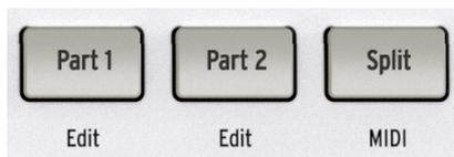
The **Part 1** and **Part 2** buttons select which part in a Multi is affected when you perform other operations such as loading a Preset or turning the [Macro \[p.32\]](#) knobs. For now, it's most important to know how they affect loading a Preset.
