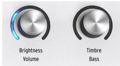
First, select a Part. Then, hold **Shift** and turn the **Brightness** knob to adjust the volume; turn the **Timbre** knob to adjust the panning.
