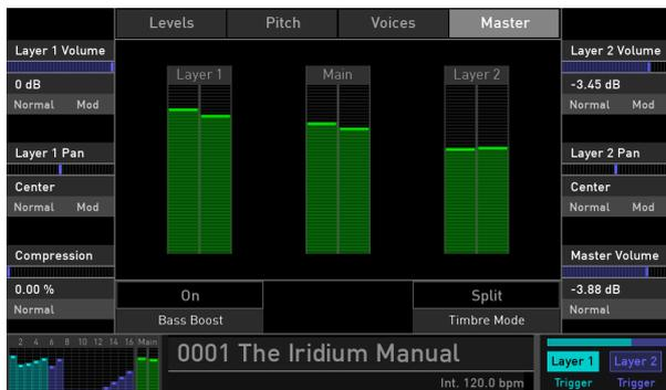
The current volume of Layer 1, 2 and main volume is displayed in the gain meter representation.
