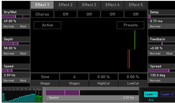
⚠ For the typical Chorus effect sound the **Dry/Wet** parameter should be set to 50%.
