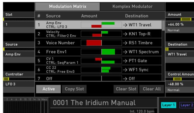
This page shows all modulation assignments in a list. You can set up to 40 assignments.
