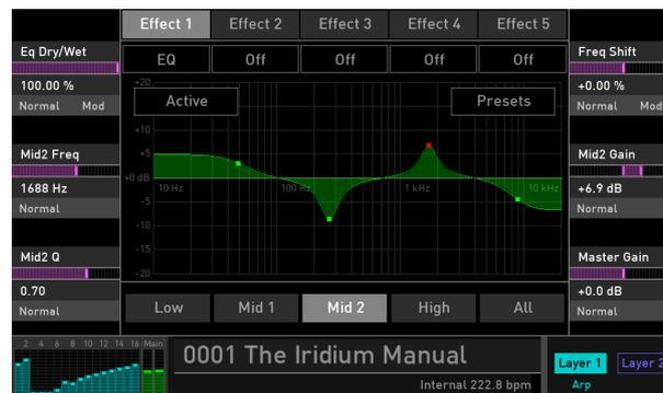
! Tap on the corresponding EQ curve in the touch-screen display to edit the **Frequency** and **Gain** parameters.
